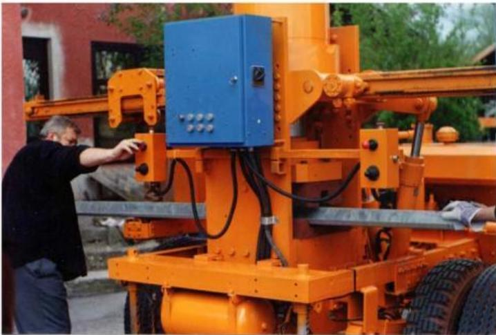
yard operated in Frankfort, KY. Prison labor straightens damaged or bent rail and posts using a rolling machine that can straighten the rail and posts and restore the "W" shape to the rail element. The straightened rail and posts are then picked up, regalvanized, and returned to the yard by a contract vendor.
